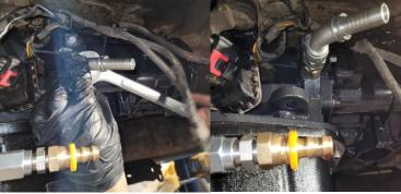
Measure and cut a section of the transmission filter hose supplied and install onto the barb fitting at the "IN" port of the filter head and secure it tightly with hose clamps. Install the other end of the hose onto the barb fitting attached to the return line from the cooler and secure tightly with hose clamps as shown.
