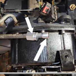
Insert the compression nut, compression ferrule and the JIC fitting (1604041) over the forward portion of the transmission line and tighten.
