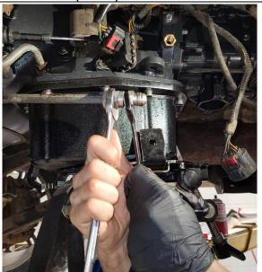
Install the straight 1/4NPT-JIC (1604048M) fitting into the open port on the transmission using pipe sealant on the threads. Thread the fitting in finger tight, and then turn once more with a wrench. Do not over torque as you will damage the case.
