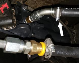
Flow direction from cooler to the filter and from the filter to the transmission case.
