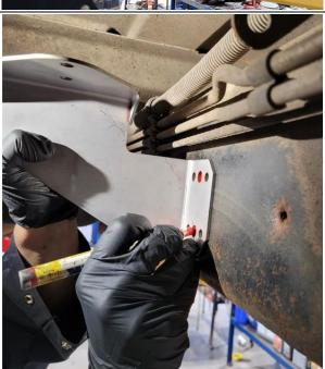
To allow for easier drilling, center-punch the two marked spots for the mounting bolts. Using a 5/16" drill bit, drill pilot holes for thread cutting mounting bolts. Make pilot thread using supplied thread cutting bolt on the two holes as shown.
