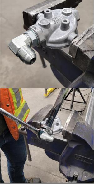
Install the **#8 JIC female fitting x ½" hose** barbed fitting (1604047) into the **90° ORB fitting** (1604046) as shown.
