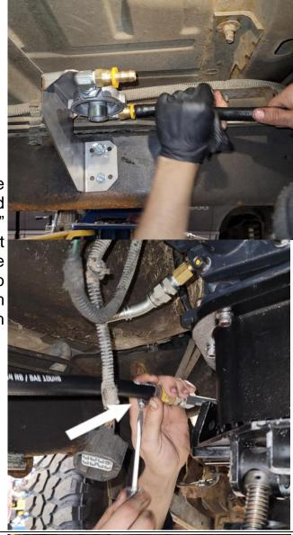
Measure and cut a section of the transmission filter hose supplied and install onto the barb fitting at the "Outlet" port of the filter head and secure it tightly with hose clamps. Install the other end of the hose onto the 45° barb fitting placed on the transmission secure tightly with hose clamps as shown.
