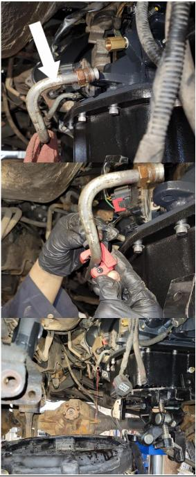
Clean the ends of the cut pipe and then discard the short portion and fitting from the transmission side.
