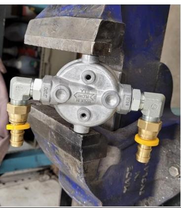
Position the filter head on the filter mounting bracket and install the 2 bolts using the flat washers supplied.
