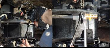
Thread the 45° JICF to ½ Hose barb fitting (1604049) in place. Align the hose inlet correctly and tighten with a wrench, use a second wrench to hold the NPT(1604048M) fitting.
